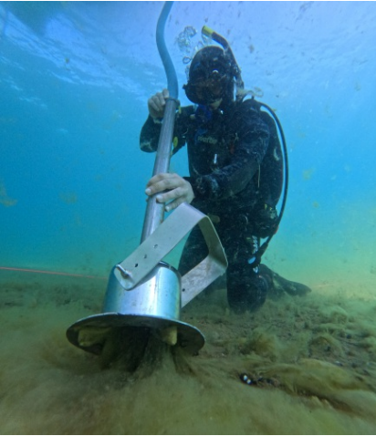
UC Davis research diver removes metaphyton from Tahoe's lake bed using surface supported suction removal device.
