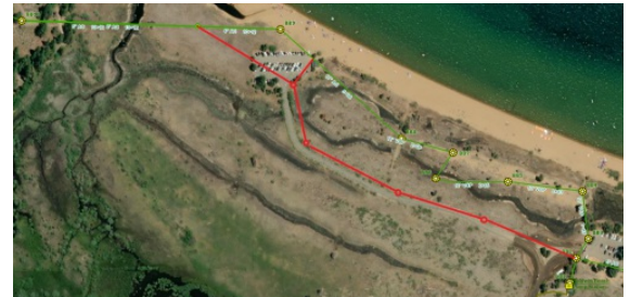
Proposed project relocates 2200 LF of gravity sewer main, which is currently located within SEZ to paved area and compacted road shoulder. Reduces risk of sewer discharge directly to Lake Tahoe.
