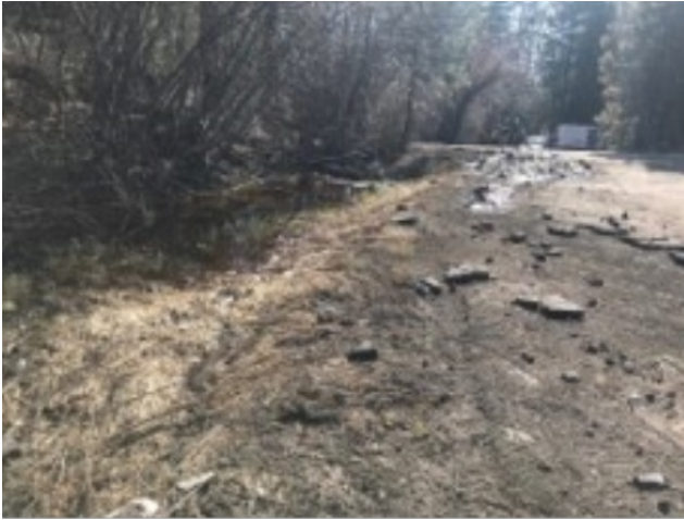
Traction abrasive and broken asphalt extend into the tributary of Edgewood Creek
